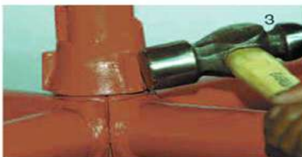
3 Rotate the top cup with hammer to lock the blade ends
