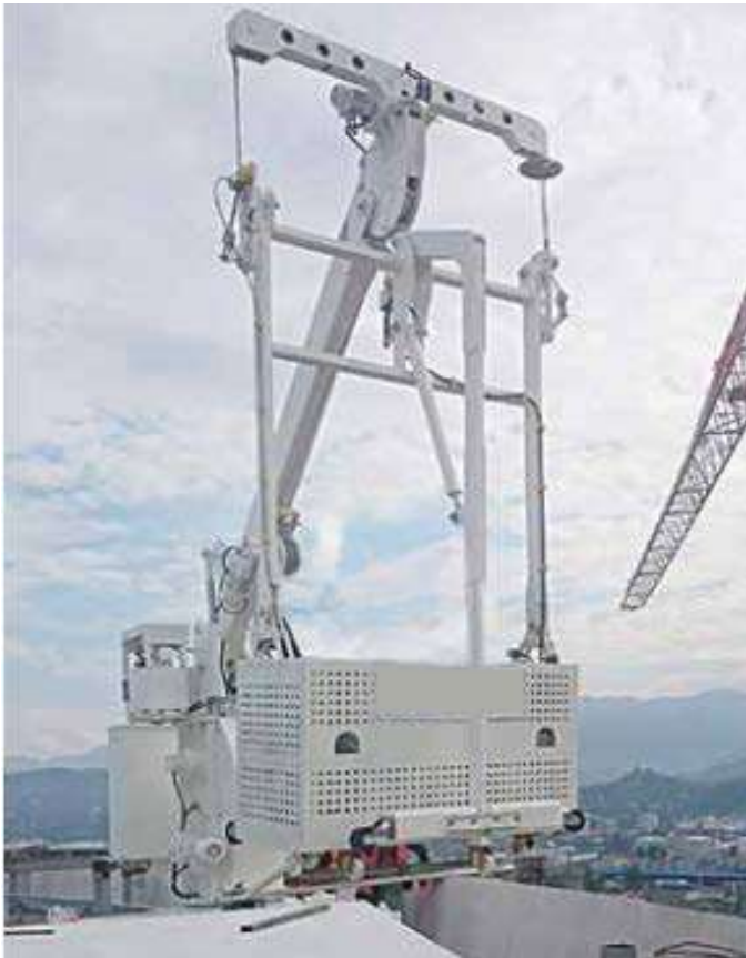
Roof machine with Pantographic Cradle
